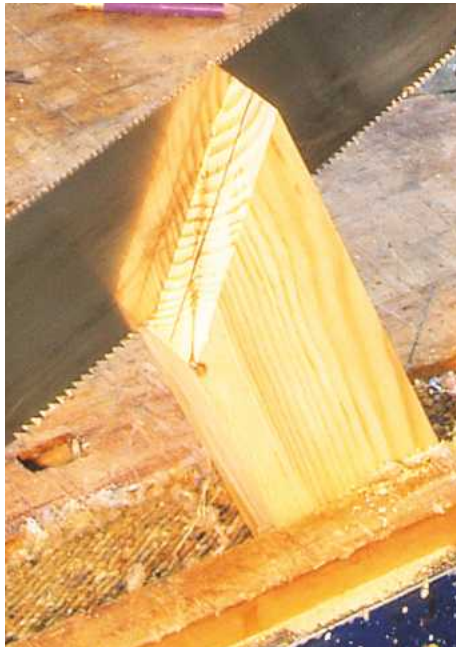
▲ Pic.4 For the bridled mitre remember to mark the saw cuts from the same face
